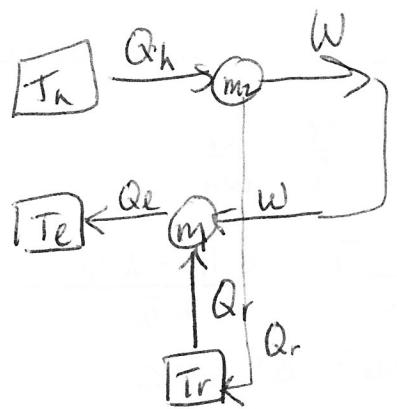
5. Thermal Pollution. A river with a water temperature  $T_e = 20^\circ\text{C} = 293\text{K}$  is to be used as the low temperature reservoir of a large power plant, with a steam temperature of  $T_h = 500^\circ\text{C} = 773\text{K}$ . If ecological considerations limit the amount of heat that can be dumped into the river to 1500 MW, what is the largest electrical output that the plant can deliver?
