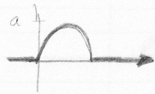
$$x(t) = \int_0^{\pi/\omega_1} \frac{m}{m\omega_1} a \sin \omega_1 t' e^{-\beta(t-t')} \sin \omega_1 (t-t') dt'$$
